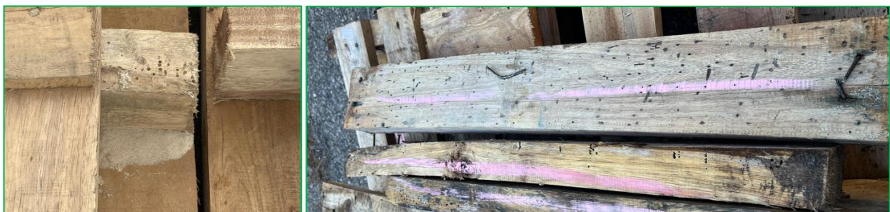
Images: Evidence of boring dust and galleries in infested pallet wood created by conifer auger beetle.
